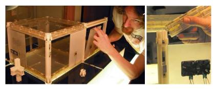
Figure 2. House\_n pultrusion chassis and communication: 1/12th scale model of a post and beam chassis to study embedded computational technology that allows newly-introduced devices to announce their presence on the network (McLeish, 2003).
