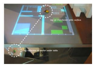
Figure 12. Digital table (Stigge 2000), with a design iteration interface (McLeish 2003). A video projector below projects an edge-to-edge image, reflected off an angled mirror. A camera below can be used for computer vision tracking of objects with unique LED patterns above.
