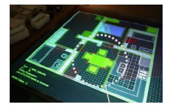
Figure 17. Plan view of a proposed design, showing how a computational critic evaluates the relationship of the dining area and the kitchen with respect to access and privacy (Williams 2003).
