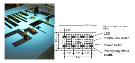
Figure 13. Left: optically tagged object bases before the model covers are applied. Right: LEDs at base of each object that provide a unique pattern for computer vision recognition of identity, location, and orientation (McLeish, 2003).
