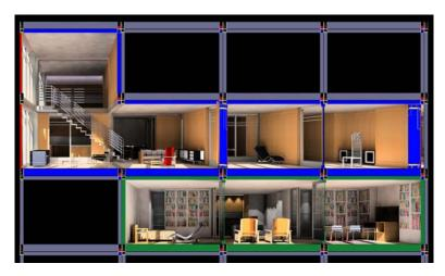
Figure 4. House\_n volumetric chassis/infill building section showing loft modules and two possible apartment infill solutions. Upper apartment is a five-bay unit with wood-veneer cabinetry. Lower apartment shows a three-bay "Ikea-like" fit-out (Rendering: Larson 2003).
