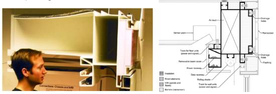
Figure 1. House\_n pultrusion chassis: full-scale model (left) and detail drawing (right) of a prefabricated pultrusion chassis showing beams, column, connectors, raceway for power and data, attachments for exterior wall and floor, housing for equipment, exterior insulation, and linear diffuser (Lawrence, 2002).
