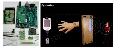
Figure 7. "Tini" micro-controller and one-wire sensors installed in each PlaceLab infill component, and wireless, wearable House\_n MITes (MIT Environmental Sensors) communicating accelerometer, location, and identity data to receivers located in either PlaceLab I3 components or wearable PDAs (Mungia Tapia 2004).
